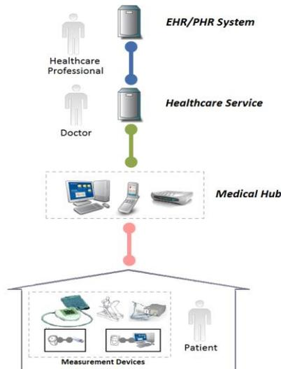
**Fig. 1.** Architecture of an RPM system
